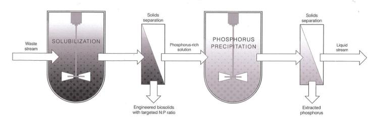
STAGE 1: Treat the centrate/filtrate to solubilize any phosphorus that is not already in solution. The separated manure solids, which contain little to no phosphorus, are suitable for land application.
